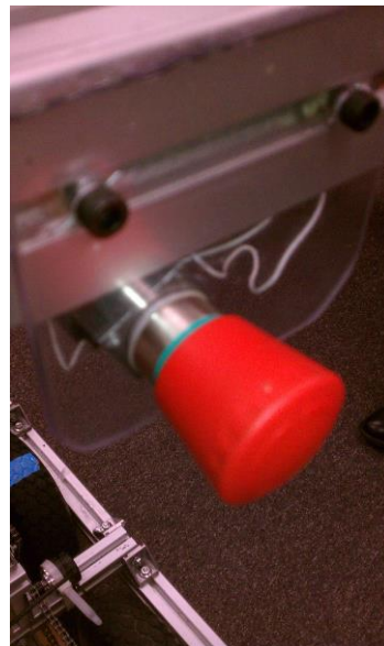
Figure 3. Manual emergency stop
